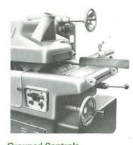
**Grouped Controls** All controls are grouped adily to hand for quicker and safer operation.
