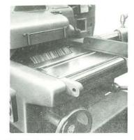
Idle Roller Bed Allows stock to be fed up to fence for easier feeding and less operator fatigue.
