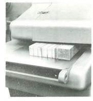
Grooving Both splitting and grooving can be done in one pass, giving increased production.
